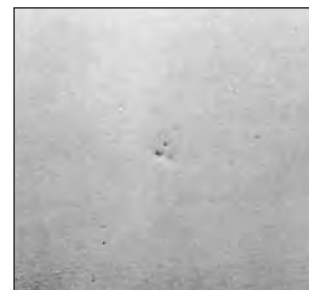
Pinhole texture by inappropriate rust proof.
