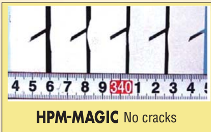
● Penetrant indication after Y-groove weld cracking test
