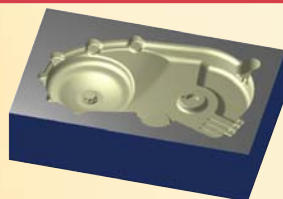
Simulated mold 130 × 300 × 480 (mm)
